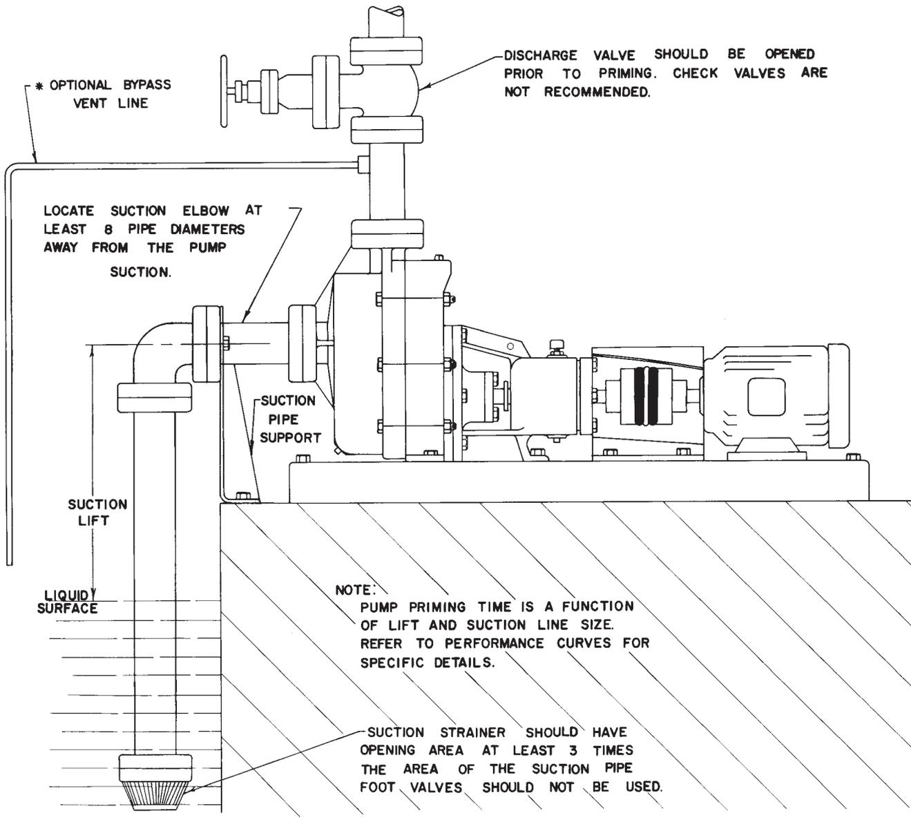
\* IF A CHECK VALVE IN THE DISCHARGE IS NECESSARY OR IF THE DISCHARGE REMAINS FULL AT A LOW POINT (FLUID TRAP) DURING PUMP SHUT DOWN, A BYPASS LINE MUST BE RUN FROM THE PUMP DISCHARGE (BEFORE THE CHECK VALVE OR FLUID TRAP) BACK TO THE LIQUID SOURCE; OTHERWISE THE PUMP MAY NOT PRIME.
